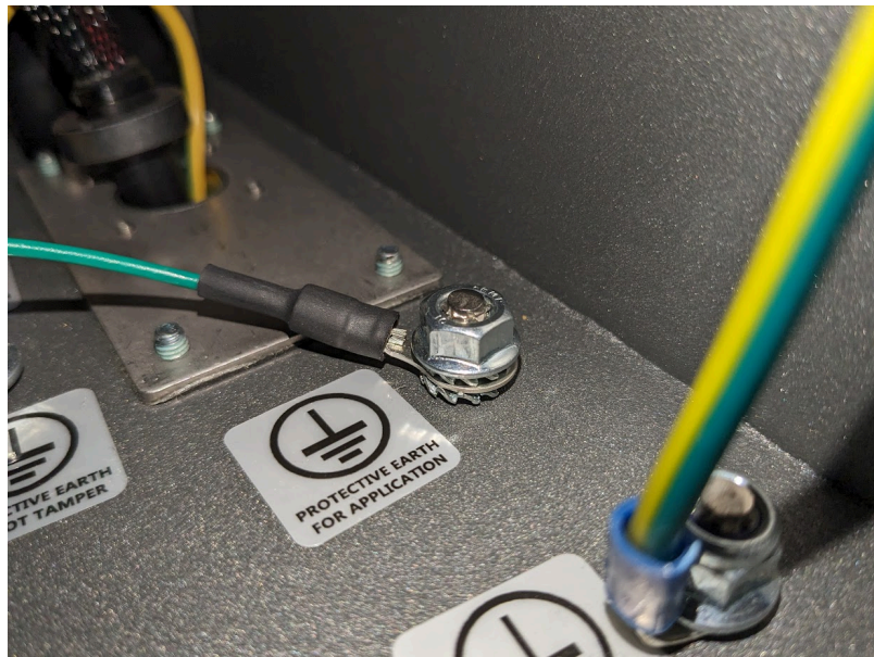
Fig. 3-16: Example of Ground Connection in Robot Control Box
