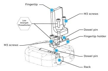
Fig. 3-8: Mounting fingertips on holders, and holders on racks.
