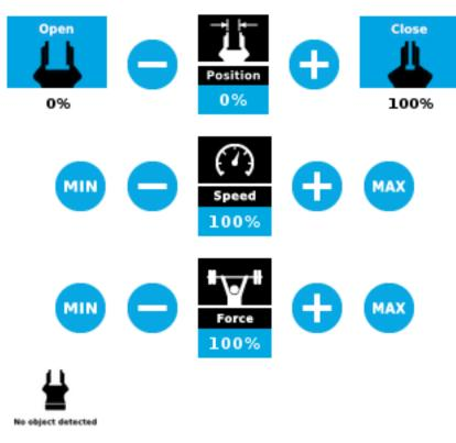
Fig. 4-24: Gripper Toolbar After Activation
