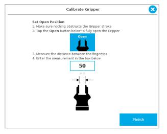
Fig. 4-18: Second step of the calibration wizard
