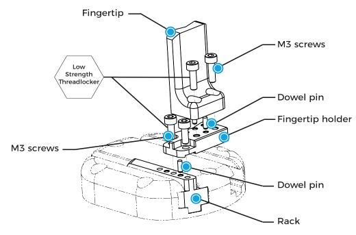
Fig. 1-3: Mounting a fingertip on a fingertip holder (example).
