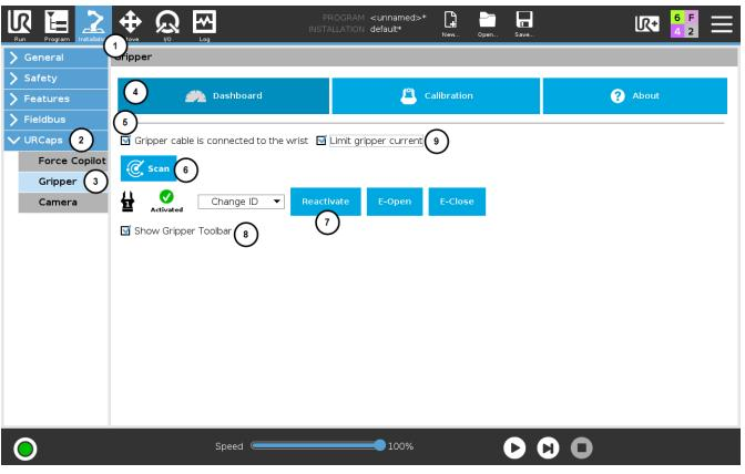
Fig. 4-8: Gripper Dashboard (steps highlighted)
