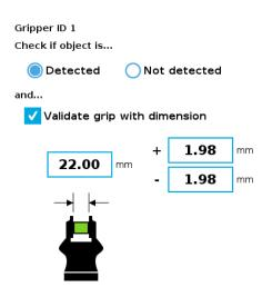
Fig. 4-27: Grip Check node interface with dimension validation
