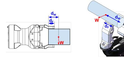
Use the following equation to calculate th maximum load if the center of gravity of the object is not centered in between the finger pads.
