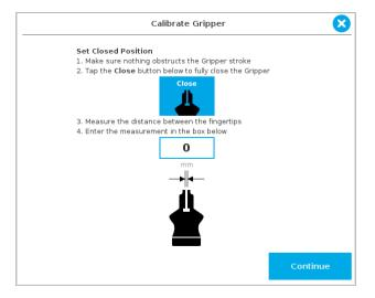
Fig. 4-17: First step of the calibration wizard
