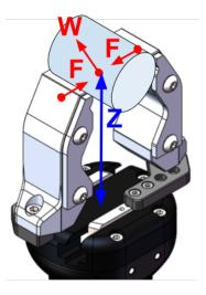
The maximum load force W depends on the distance Z (on the Z-axis) at which said force is applied at finger attachment.
