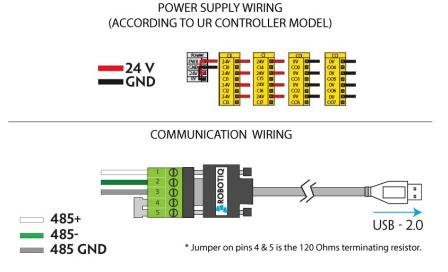
Fig. 3-12: Hand-E Gripper wiring to Universal Robots controller.
