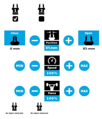
Fig. 4-25: Gripper Toolbar (expanded, multiple grippers)
