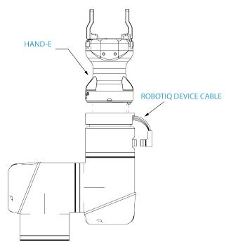
Fig. 3-15: Robotiq Hand-E with device cable wiring scheme
