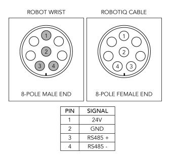
Fig. 3-16: Pinout of the Hand-E cable-to-wrist coupling
