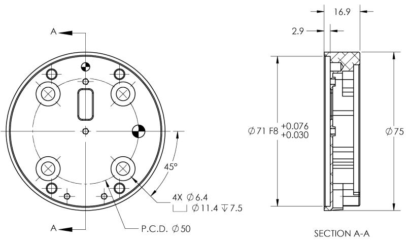
Fig. 5-3: Coupling for ISO 9409-1-50-4-M6.
