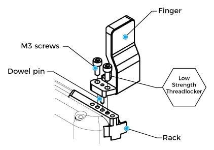
Fig. 1-2: Mounting a finger on a rack.
