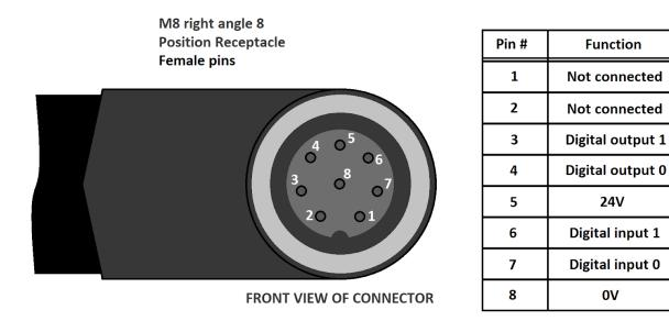
Fig. 3-14: Pinout of the I/O Coupling
