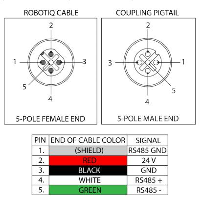
Table 3-4: Pinout of the Hand-E Gripper pigtail and device cable.
