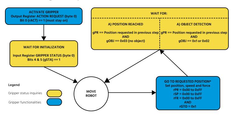
Go to requested position is used to open/close the Gripper until a contact with the object is detected, or the requested position is reached.
