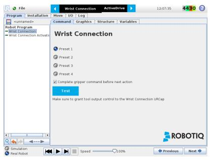
Fig. 4-5: Wrist Connection Node Interface.
