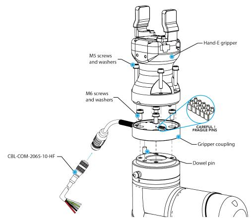
Fig. 3-1: Installing Hand-E on the robot tool flange for CB-Series.
