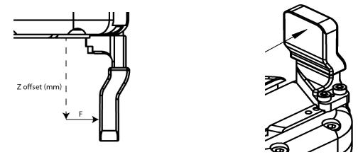
Fig. 5-11: Z-axis offset at which force/payload is applied.
