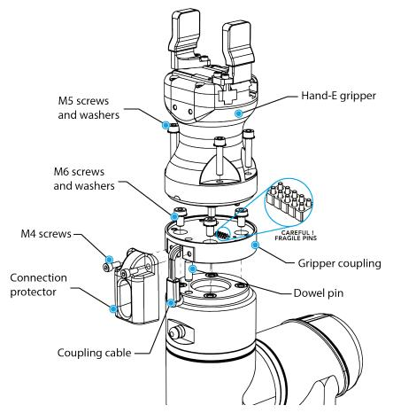
Fig. 3-2: Installing Hand-E on the robot tool flange for e-Series.
