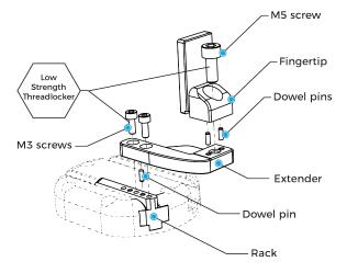
Fig. 3-9: Mounting extenders on fingers, and extenders on racks.
