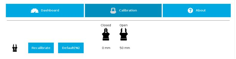
Fig. 4-19: Single Gripper, calibrated
