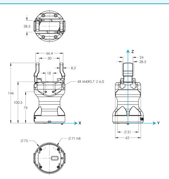
Fig. 5-1: General dimensions of Hand-E (open) with flat rubber (NPR) overmolded fingers.
