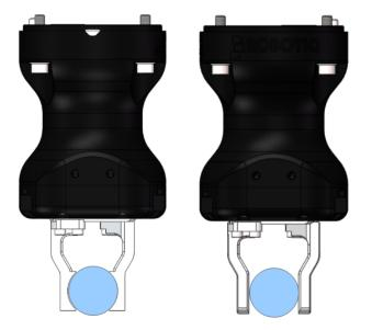
Fig. 5-10: Form-fit grasp (left) and friction grasp (right).
