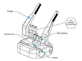
Fig. 3-10: Mounting bin picking fingers on racks.
