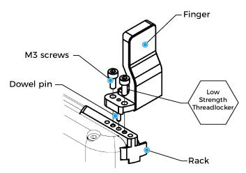
Fig. 3-7: Mounting fingers on racks.
