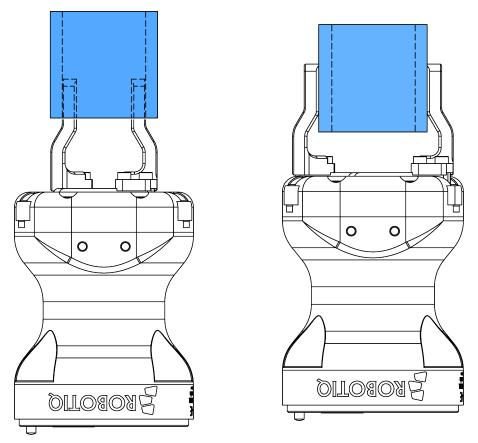
Fig. 1-4: Hand-E Gripper internal and external gripping.
