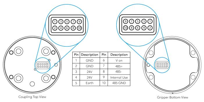
Fig. 3-11: Pinout to the Hand-E Gripper cable-to-wrist coupling.
