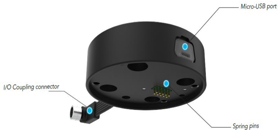
Fig. 3-3: Robotiq I/O Coupling
