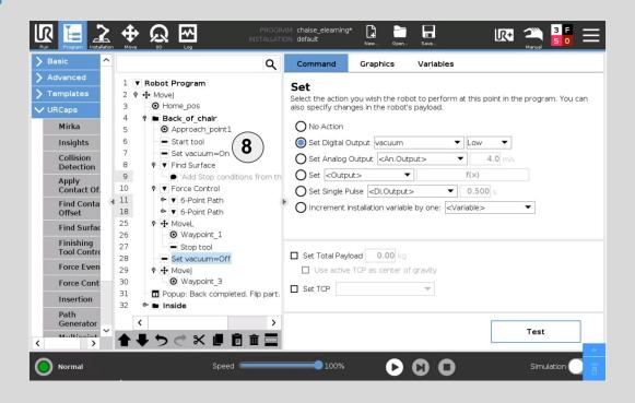
8 The Start tool and Set vacuum commands are used before touching the surface.
