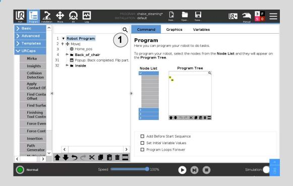
1 Robot Program is the section of the program where the main loop of the program is located. In our case, we are not using a **Before Start** sequence, but it may be useful if you have variables to set for instance.
