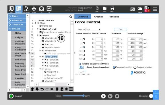
The **Inside** folder processes the inside of the chair. The whole process is exactly like the back of the chair, but with 3 **6-Point Path** nodes instead of 2.
