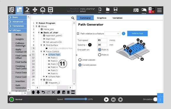
11 The **6-Point Path** is used to generate the trajectory required to process the surface.
