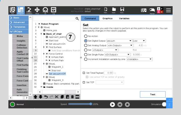
7 The Approach Point is set over the first point of the Path Generator.
