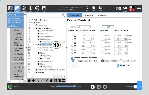
10 The Force Control node is used to apply the proper force when processing the surface. Most of the time, the force will be in the +Z direction of the tool reference frame.
