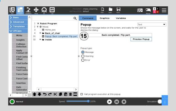
15 In this example, a **Popup** is used to let the operator know that the back of the chair is done. Once the setup is changed, the operator can continue the program through the teach pendant.
