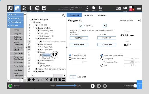
A linear relative move is added after the **Force Control** node. It moves in the -Z direction in the tool frame of reference.
