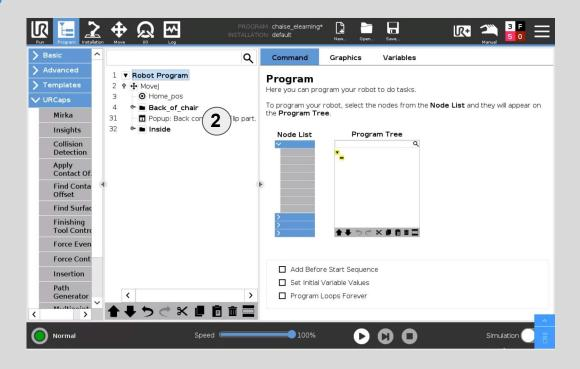
2 Folders are used for the different sections of the part. Here we use one for the Back of the chair and another for the Inside of the chair.
