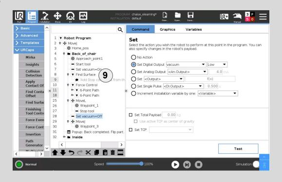
9 The **Find Surface** node is used to contact the surface before the **Path Generator**.
