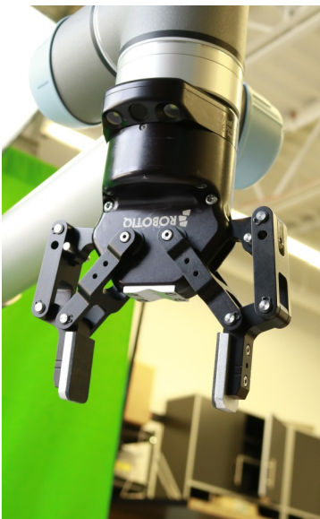
Robotiq Wrist Camera with integrated lighting
