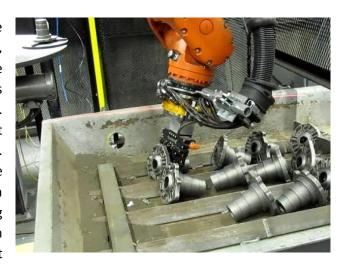
depending of its configuration. Paired with a vision system, the gripper knows where the part is and what its configuration is. The robot controller/program can then analyze the different scenarios it was taught and respond with a motion according to these scenarios.
