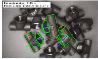
different, you want to have a gripper that can grip it all. As you can see in the picture, the vision system is able to figure out what the orientation of the parts is, although your set up might not allow you to pick the part as you might want to. With a self-adaptive gripper, you can have a couple of options for the same scenario compared to other grippers that have only one way to grab the object.
