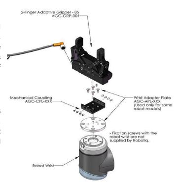
coupling should be bought for your robot and how to install it. We are currently manufacturing kits for <u>Baxter</u> and <u>Universal Robots</u> for our <u>2-Finger Adaptive Gripper-85</u>. This makes the integration easier for people that are using our Gripper with these robots.
