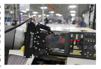
To know what type of protection you need, the IP Rating is a good way to quantify this. In fact, the different ratings will help you monitor your application and determine your needs. All Robotiq Grippers are rated IP 67 which means that they are "dust-tight" and that they are protected against water penetration from 1 to 30 minutes.
