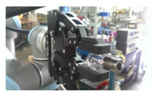
gripping surface can be adapted to reduce the impact on fragile part surfaces, thus <u>force-controlled grippers</u> can also be part of the solution.
