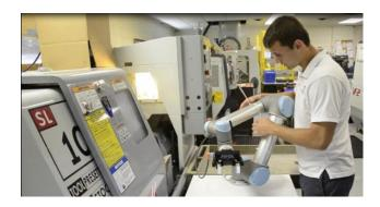
At the time they started to automate the process, they decided to go ahead with a conventional workcell, fully guarded, that cannot easily be reprogrammed for their needs. The current pneumatic grippers are limited to a few parts, and since Inertia Switch makes over 1,000 parts, they needed a more flexible solution to optimize their machine tending production process.
