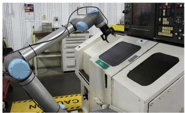
optimized to reduce cycle time. For example, if an object is 25mm wide, it is possible to open the Gripper to 30 mm to grab hold of the object. This means that the Gripper only has to perform a 5 mm stroke instead of a 60mm stroke during the grasping operation. And the same thing occurs once the object is released. These specifications mean that a couple of seconds are saved by each pick and place operation which at the end of the day will result in a reduction of cycle time.
