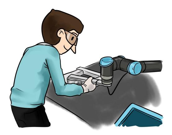
The "record trajectory" function makes it easy to teach motions for finishing or polishing. You can even use the sensor's data to make sure a constant force is applied onto the surface while the motion is performed. That way, you'll maintain the right amount of contact between the tool and the surface. Just make sure you confirm that your sensor includes this feature before you start!
