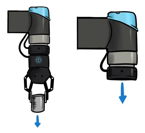
When a force sensor is mounted on an end-effector, all forces applied to this gripper or tool will be sensed by the sensor.
