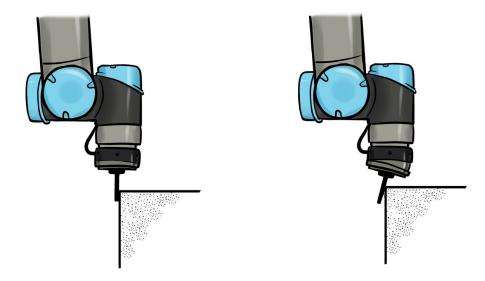
Depending on the sensor's stiffness, certain forces can cause the part to shift its orientation (see the figure above). This shift might make the task harder to accomplish. Do yourself a favor and verify that the stiffness of the sensor you're considering will not lead to such undesirable situations.
