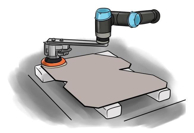
A UR10 (robotic arm) combined with an <u>FT 300 (Robotiq force torque sensor)</u> was able to take over part of the operator's work. Now the two of them – human and robot – work together with greater productivity.
