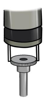
First, with the gear held securely between the gripper's fingers, the robot should move towards the shaft until it reaches it.
