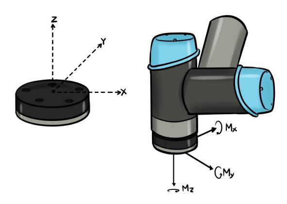
Sensing range tells you the range of forces and torques that the sensor is able to read. (Some sensors can only read forces, whereas others can read both forces and torques; forces are given in Newtons or pounds, and torques in Newton-meters or foot-pounds.)
