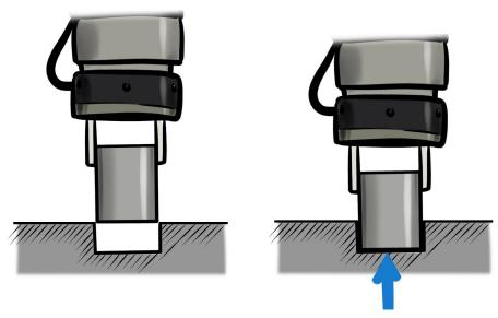
The first step of a part-insertion application is programming the robot to move downwards until it makes contact with a surface. If it hasn't reached the bottom of the insertion area, the robot should adjust its position laterally until it senses a drop in contact force.
