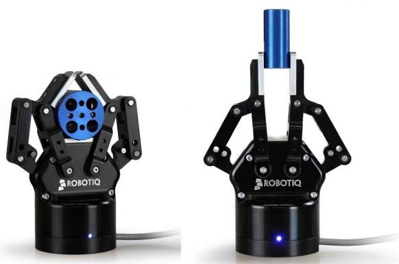
Underactuated adaptive fingers allow for a parallel or encompassing grip.
