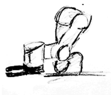
Adapter plate for changing the gripper's orientation or offsetting its position.
