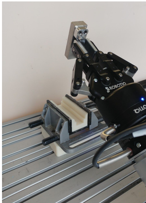
Gripper unable to flip a part.
