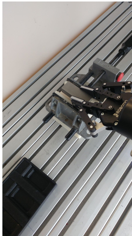
Use of a fixture to flip the part.
