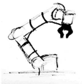
Cable management: not enough excess cable.
