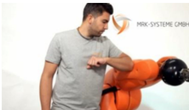
Example of the smooth, “soft impact” design of a collaborative robot
