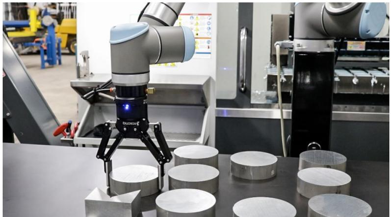
One problem remained: He knew he needed either a vision system or a conveyer, to pick up the raw parts from the table. "Everyone told me that it's a very difficult process, that you need to have a person in your shop to do it", Caughey recalls. A big plus when using a robot is the ability for it to continue production during unattended hours in the shop. This of course increases productivity since twice as many parts can be made in the same time.
