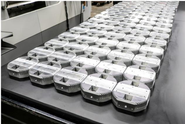
Since WALT Machine Inc. bought its robot, named Arthur, twice as many parts are being machined everyday. The CNC machining still takes the same time, but it's the number of operational hours that make all the difference. The company was able to save half the time in production by eliminating a lot of machine idle time.
