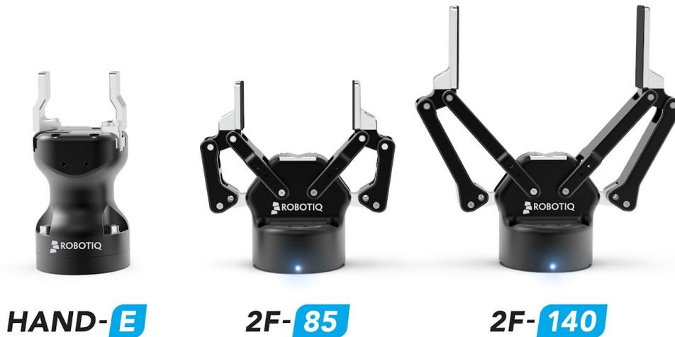
Your gripper is the robot's "hand," but it's not nearly as versatile as your hand. Grippers work best when parts have at least two parallel surfaces. The stroke of the gripper will limit the range of parts you can handle.
