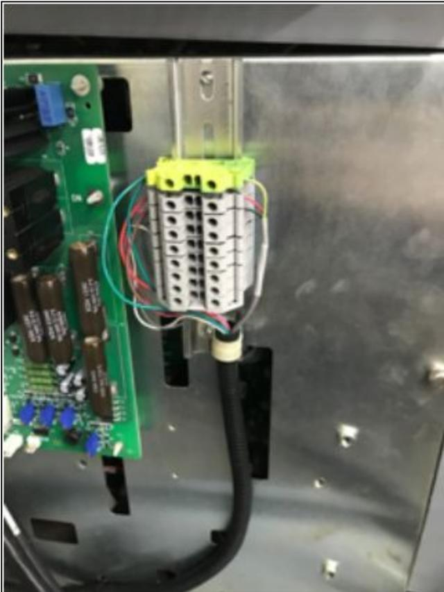
*Couple relays inside the CNC controller*
