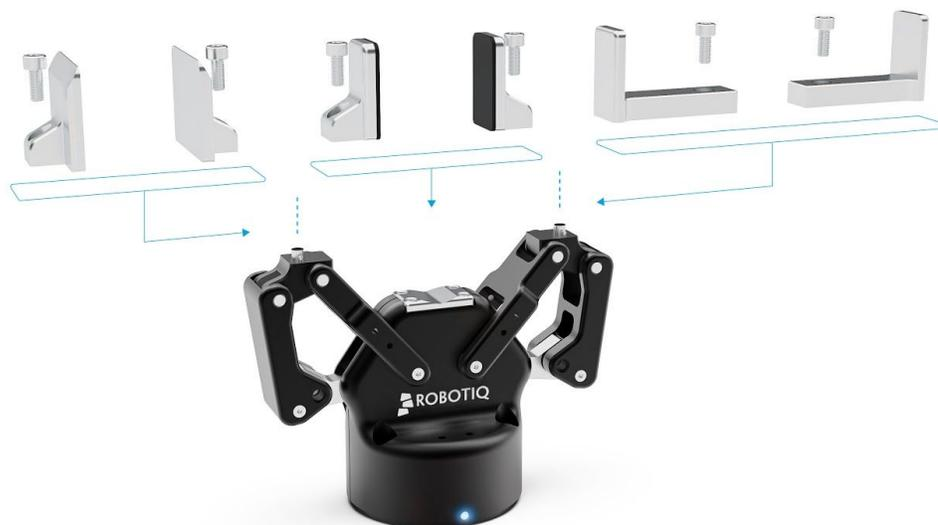
*Robotiq Gripper with fingertips designed to grasp cylinders in two different axes (as well as flat/square geometries).*
