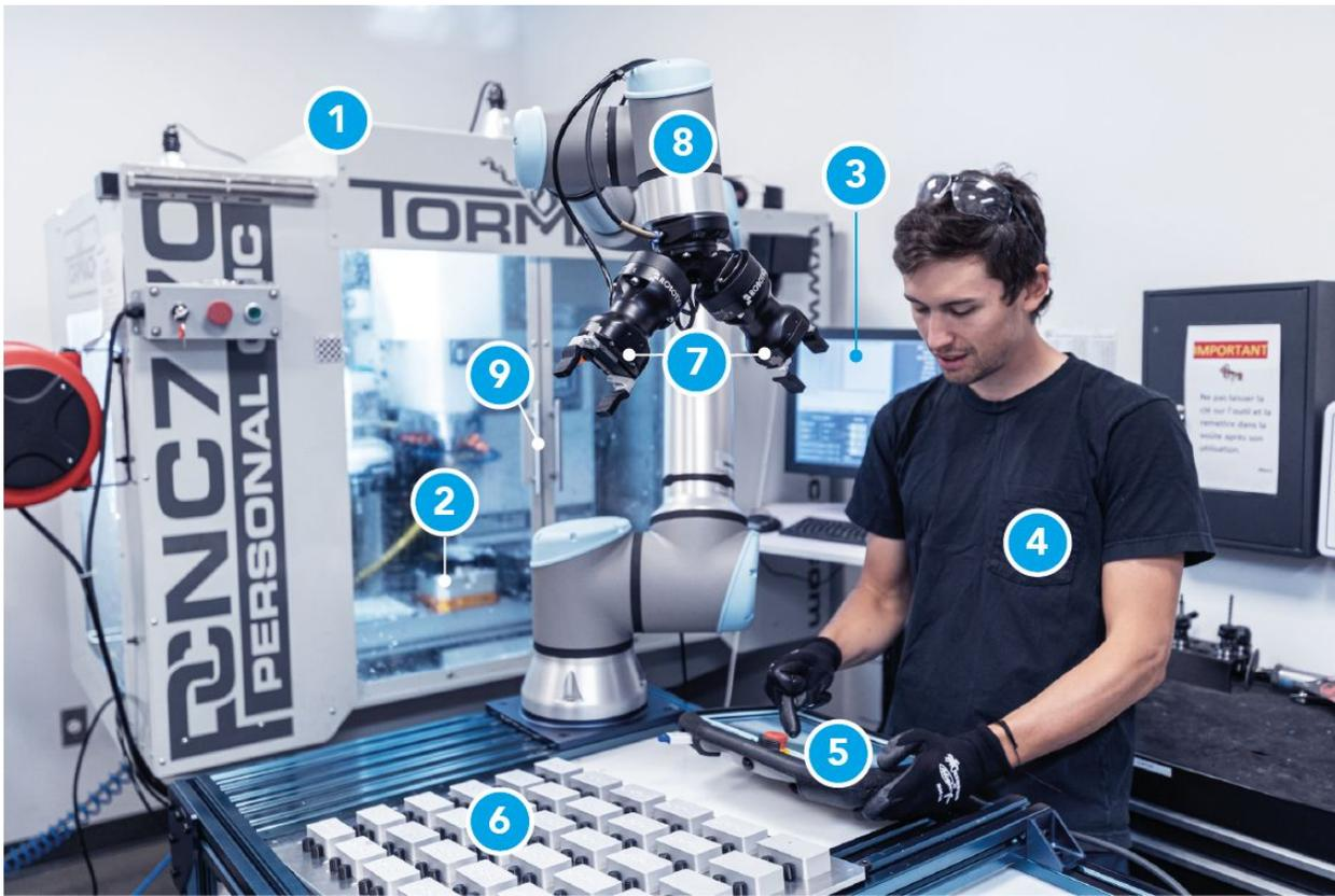
1. **CNC machine:** Autonomously machines parts (CNC stands for computer numerical control).
