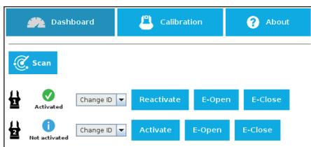
Figure 2. Activating two Hand-E grippers on the Teach Pendant.
