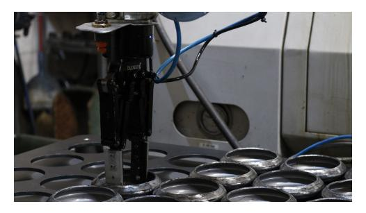
"With Robotiq 2F-140 Adaptive Grippers, we could program different positions and tailor them perfectly for each part of the process."
