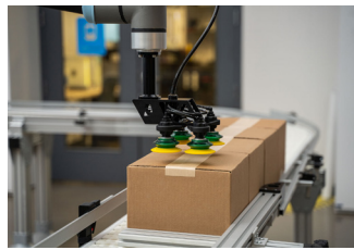
Wrist extension for vertical offset to handle smaller cases
