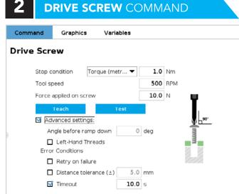
Control the screwdriver directly from the UR Toolbar to use, test or set it. Seamlessly integrate the force sensing, vacuum, cobot, screwdriver, and screw feeder. Automatically apply error-proofing functions to improve productivity and quality.
