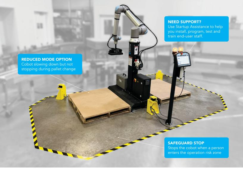
Ordering the safety package on the same PO as a PE20/AX20/AX30 will ensure safety relay and safeguard reset buttons are preinstalled. For all pricing, please refer to <a href="https://robotiq.com/price-list">https://robotiq.com/price-list</a> with the SKUs below.
