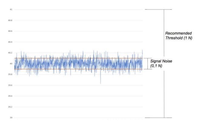
For the FT 300, as for most of the sensors on the market, the noise is greater than the resolution and that's why we spec the noise instead of the resolution (the resolution is not what limits the applications).
