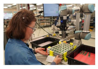
Anytime the robot has emptied all its trays, PCB testing operator Marcella Segovia receives a text message from Insights. Then she knows it's time to load new trays. They're often filled with another type of PCB, so she changes the robot program to let the gripper know which part to pick. "I was a little scared of the robots at first, but I really wanted to learn how to run them. They're fast, but I can keep up—and it's great how much we've increased our numbers. I sometimes joke that they're
