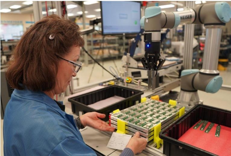
Anytime the robot has emptied all its trays, PCB testing operator Marcella Segovia receives a text message from Insights. Then she knows it’s time to load new trays. They’re often filled with another type of PCB, so she changes the robot program to let the gripper know which part to pick. “I was a little scared of the robots at first, but I really wanted to learn how to run them. They’re fast, but I can keep up—and it’s great how much we’ve increased our numbers. I sometimes joke that they’re
