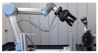
sensitivity feedback they are seeking should be measured from 3 different axes, so as not to limit the end-of-arm tool position when the force is applied.
