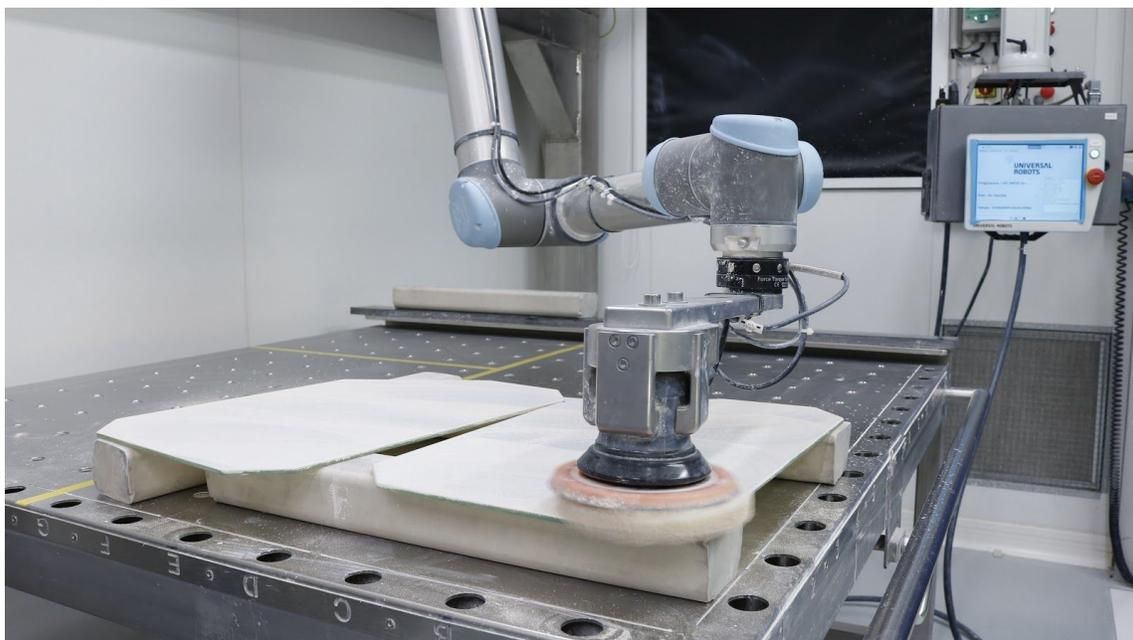
\*Robotiq recommends protecting the FT 300 Force Torque Sensor against dust
