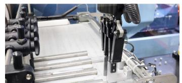
during an evening. Their KUKA robot, model KR 6 R900 is integrated with Robotiq's 2-Finger 140mm Gripper. A great benefit for Précinov is the flexibility of the Gripper, which can take parts of different sizes.
